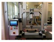
basic parameters of the process were identified, then the control-oriented dynamic model of the system was derived, and the synthesis of the PID controller was made for more precise following of the sinusoidal reference signal. Compared to hydraulic solutions that are used to achieve large forces, this pneumatic fatigue testing machine has a compact design, the desired reference is simply set via the HMI interface, it is portable, and it can be used to test materials with lower tensile strength.
