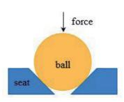
del developed by Persson. It considers the surface roughness via the two-dimensional spectral density. The model is validated experimentally by comparing the simulated leakage rates with experimentally measured values for seats with different surface roughness and anisotropy. This way, the validation shows whether the leakage model can be applied to gases.
